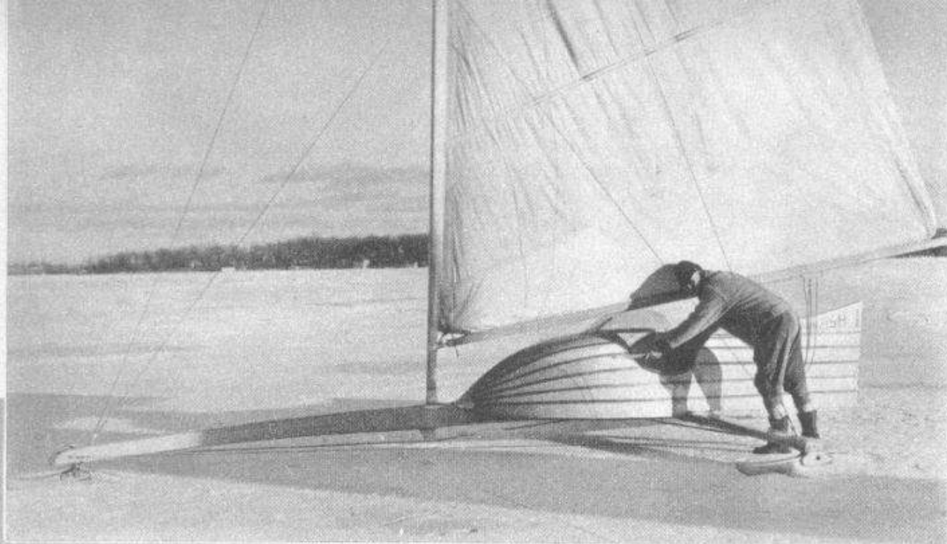
Crawfish ready for a speedy spin over the ice. The mast is braced with three sets of stays, the backbone by a martingale stay which can be seen directly below the mast.
