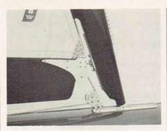
The gooseneck has a pin in it so that as you trim the 12:1 sheetrope (mainsheet), the downhaul slides down and the pin engages to prevent it from sliding up when the main is eased. In heavy wind I choose to have more downhaul, so I have a lever, which I carry in the cockpit, and use it to ratchet more downhaul on the gooseneck. In light wind I release the pin to let it slide freely, with a preventer to keep it from going up too far when the main is eased.
