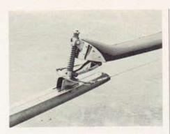
A springboard increases the length of the hull without adding much extra weight, and the spring front end fitting used to attach the springboard to the front runner allows the forward end of the boat to go down level with the aft end when the runnerplank deflects downward under pressure. Without this, when the runnerplank levels under load, the front end of the boat would be higher than the back, creating an uneven distribution of weight on all three runners.
