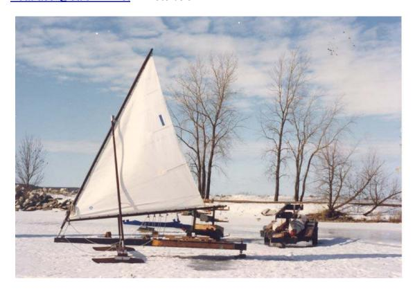
Class A, Leaping Lena, 36'10" backbone, 34'6" mast, 18'3" boom, 22' plank, 2 sets of
