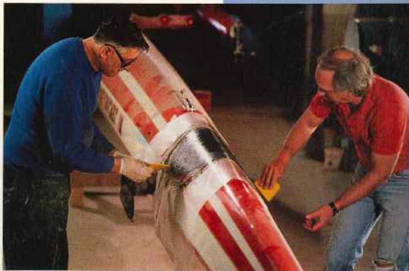
Mattison and Harken repair collision damage to Honeybucket VIII
